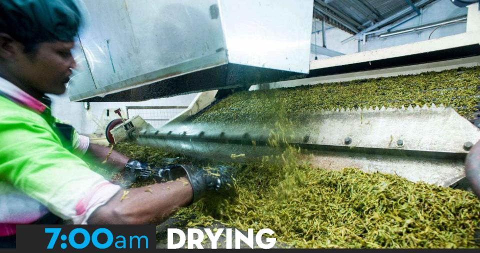
The firing takes place in a specially adapted Tea Drier machine which, at low temperature, removes all surface moisture from the leaf, rendering it suitable for the sifting and grading processes that lie ahead.
