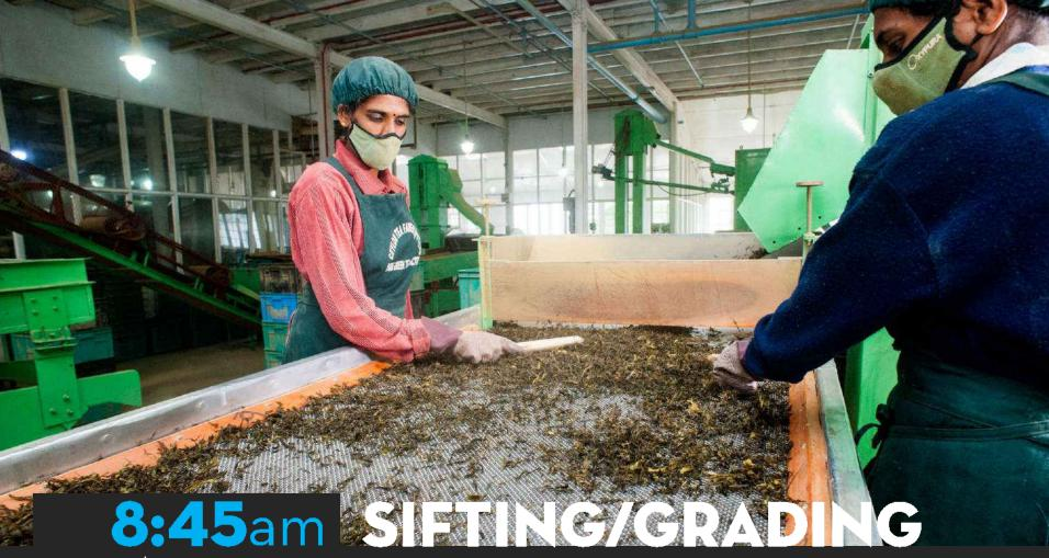
The tea is conveyed direct from the dryer to be sifted and graded. Tea particles are separated according to shape and size by being passed through a series of progressively finer meshes. The main grades are Leaf and Broken grades with the former consisting of larger and longer particles, yielding a light liquor, whilst the smaller particles produce darker and stronger liquors.
