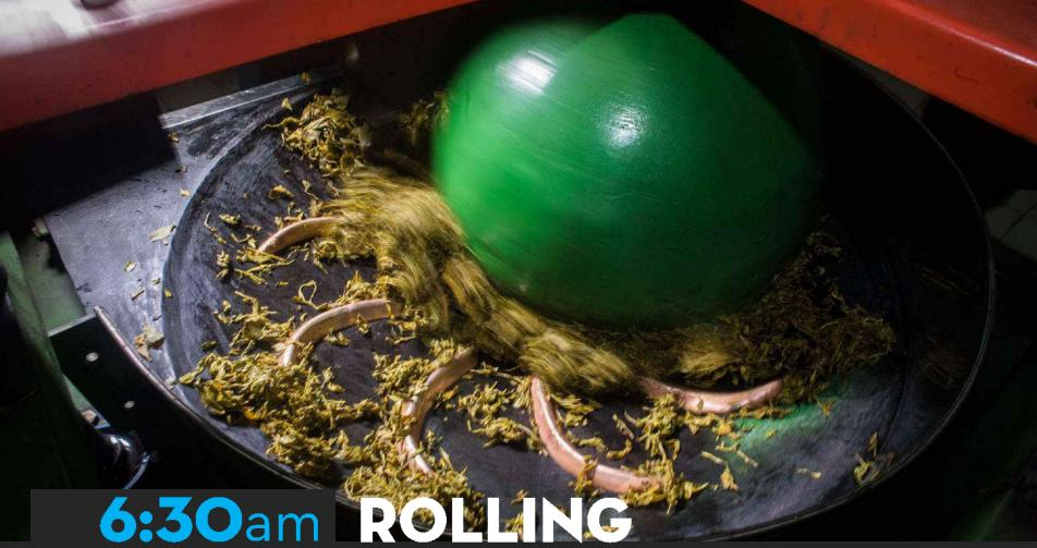
Rolling the withered leaves begins the process of oxidization by rupturing the leaf cells, allowing the cell sap to mix. In this instance, a specially made "Moon Roller", smaller than the conventional size was used.
