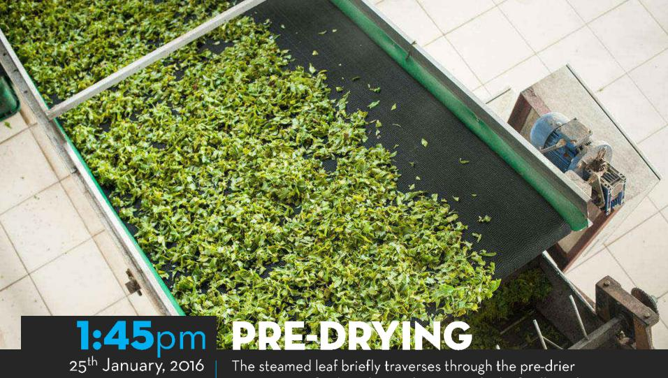
The steamed leaf briefly traverses through the pre-drier arresting any further chemical action in the leaf cells and preparing the leaf for drying in the troughs.
