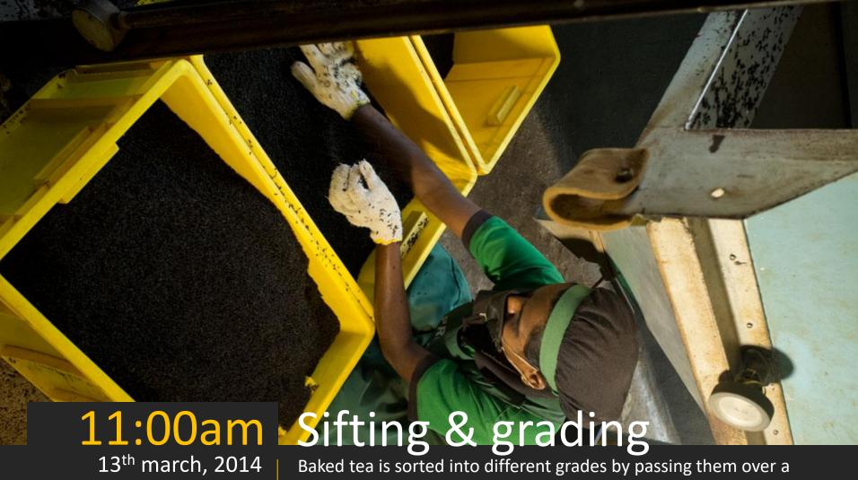
series of vibrating screens of different mesh sizes -
