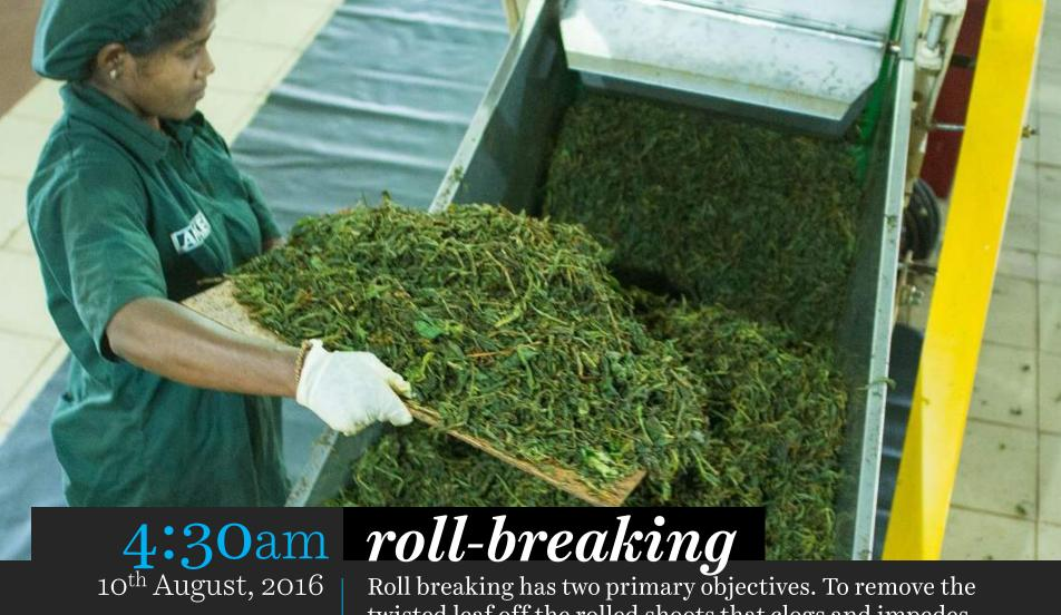
Roll breaking has two primary objectives. To remove the twisted leaf off the rolled shoots that clogs and impedes circulation, and to facilitate further twisting action on the large leaf. Additionally, it also cools the leaf which would have risen in temperature during the process of rolling.
